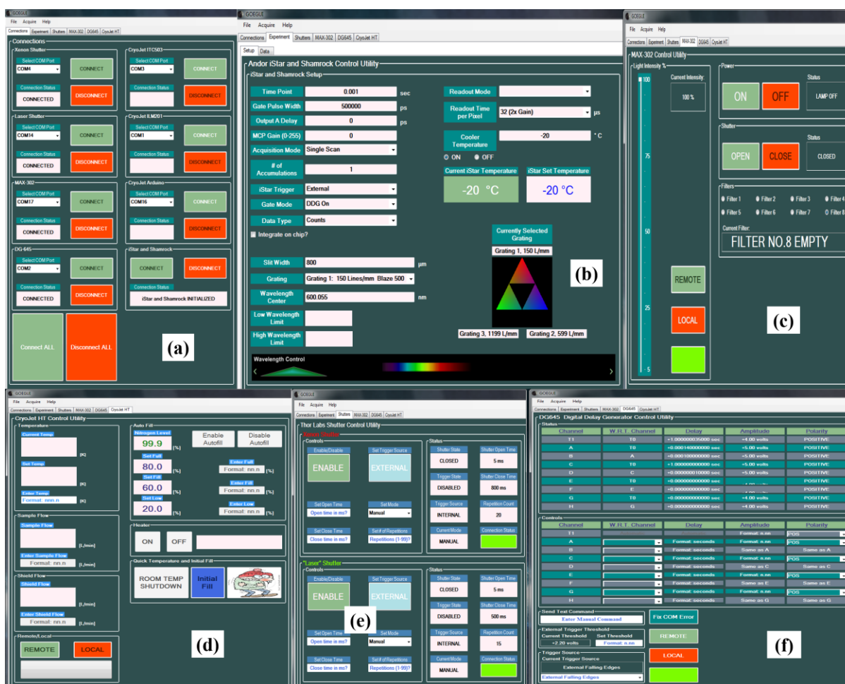
Figure 2.13. SBL2 GUI of Everything GUI (GOEGUI). (a) The connections tab where all equipment is connected to the software. (b) Experiment setup tab which configures the iStar camera and Shamrock spectrometer and defines the experimental parameters for data collection. (c) Interface for adjusting all features of the MAX-302 Xenon light source. (d) Tab providing control of the CryoJet cryogenic system. (e) Shutter tab for controlling all parameters of the Xenon and laser shutters. (f) Tab for adjusting all features of the DG645 digital delay generator.
